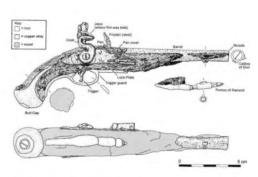
Figure 2: Illustration of pistol, identifying key terms.
